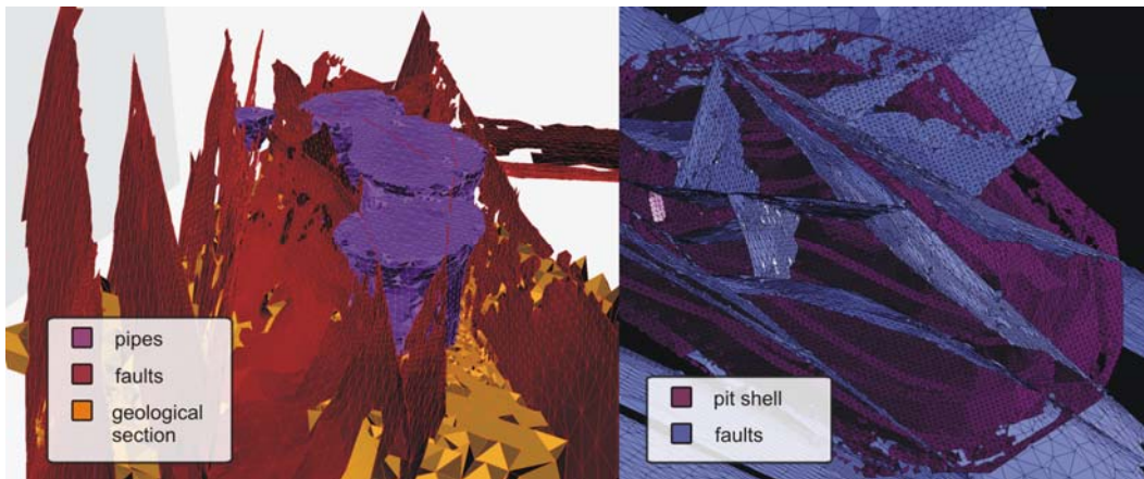
Figure 6. Example of the discretisation of some geological features in a LOP model
